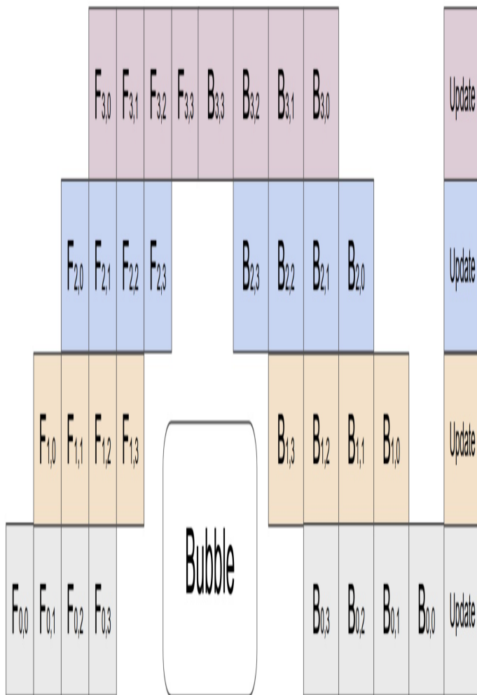
Figure 5-9. Pipeline parallelism for a neural network on 4
